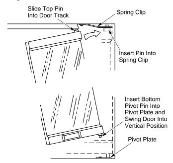
Figure 35 - Installing Optional Glass Door
